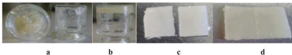
Fig. 18 (left) (a) Native damaged polymer P 1 ; (b) self-repaired polymer P 1 ; (center) (c): mechanically cut polymer P 2 ; (right) (d) self-healed polymer P 2 . 94
