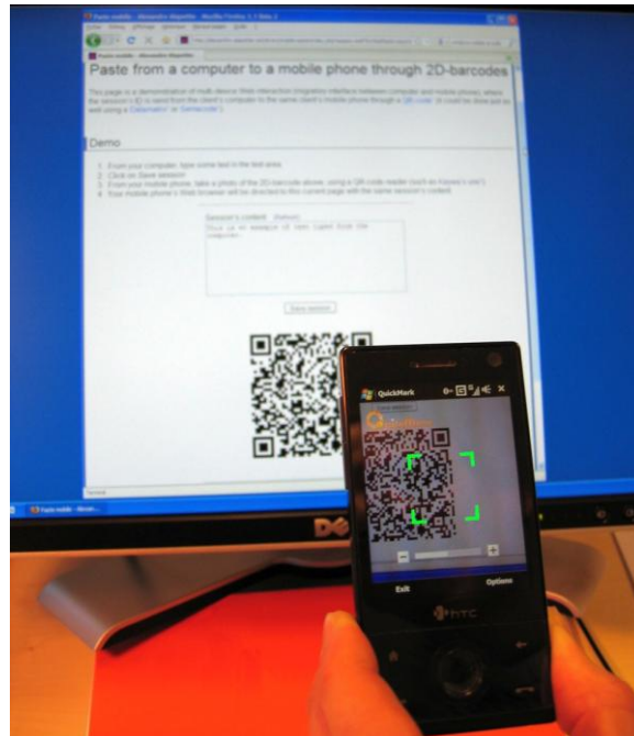
Fig. 3 A mobile phone scanning a QR-code from a Web page on a desktop computer screen, to initiate a session transfer towards the mobile phone Web browser.
