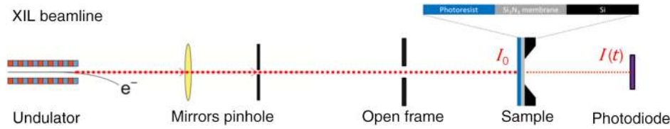
Fig. 2 Schematic of experimental setup for absorption measurements.
