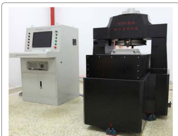
Figure 4 Ultra-precision flycutting machine tool for KDP crystal machining
