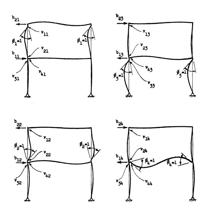
Figure 7. Matrix Elements  $b_{il}$  and  $v_{kl}$
