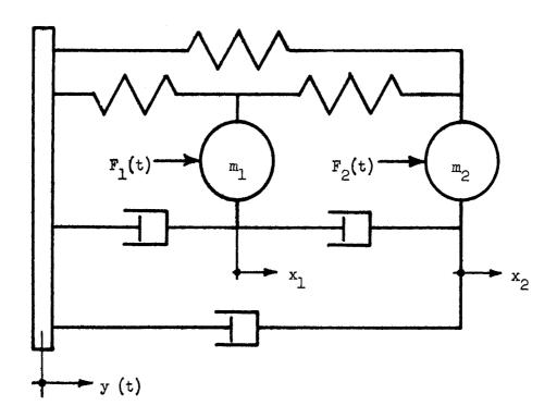
$\mathbf{x}_1$  and  $\mathbf{x}_2$  are displacements relative to base y is displacement of base
