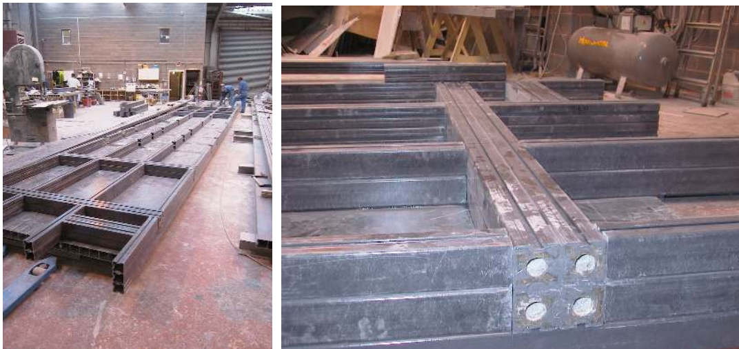
Fig. 3. Fabrication of the GFRP bridge deck, showing the configuration of the transverse beams.
