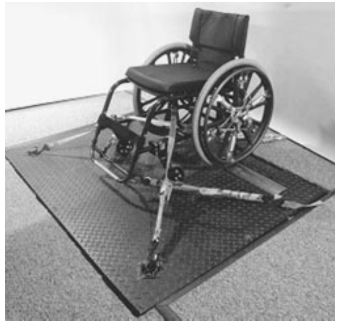
Figure 1. Wheelchair with SMART Wheels attached to the wheelchair dynamometer.
