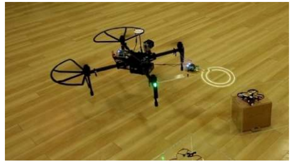
Fig. 17. Photograph of the wireless charging drone.
