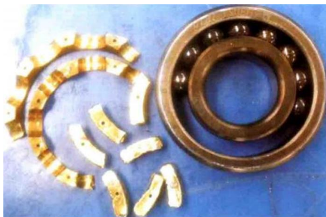
Fig. 1 Fracture failure of rolling bearing cage of aero-engine [4]
