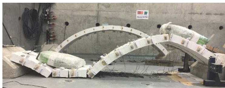
Figure 9: Masonry arch specimen after collapsing due to increasing horizontal settlements of the right support.
