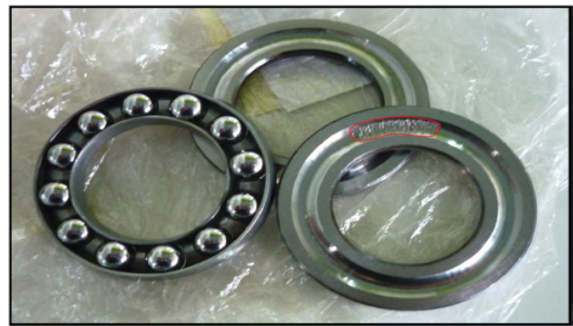
Fig. 3. Thrust bearings single direction (SNR 51207), with the spalling highlighted.
