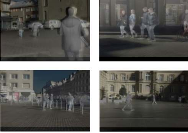
Fig. 3. Examples of synchronized pairs of visible and far-infrared images using the infinite homography registration. People close to the stereoscopic system are not well synchronized, people far from it are well synchronized.
