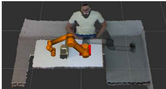
Fig. 6. The state where the UR5 manipulator is transparent is the start pose, as the state where the manipulator is orange is the goal pose.
