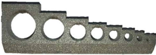
Fig. 3 Test artifact with different diameters of horizontal holes (from left: D10, D8, D6, D5, D4, D3, D2, D1 in mm)
