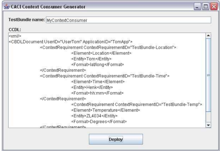
Figure 5-30 GUI of the context consumer generator.
