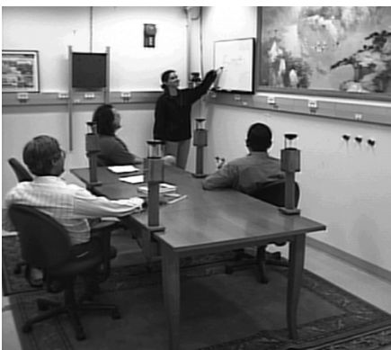
Fig. 20. Configuring AVIARY in an Intelligent Meeting Room. People are tracked, identified, and classified as presenters or participants based upon dynamic analysis of the visual and audio signals. A summarization module maintains a record of all state changes in the system which can be accessed at a later time.
