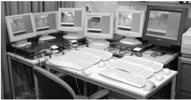
Fig. 7. Workstations that perform synchronous grab from multiple cameras.
