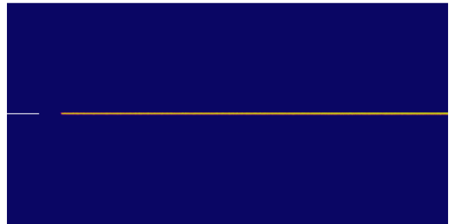
Fig. 12 Crack propagation in a constrained path configuration with \Delta U = 0.05 mm. Branching is completely suppressed, dissipation takes place only inside the middle interface and the crack accelerates up to the Rayleigh wave speed.
