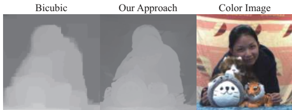
Fig. 6 Comparison between our method and bicubic upsampling on real scenes. The disparity map is upsampled from 320 \times 240 to 640 \times 480 . Our method preserves sharp edges and maintains smoothness, which is critical to reliable DoF synthesis.
