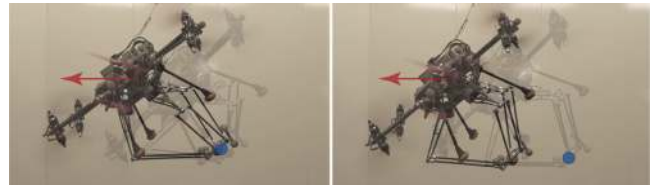
Fig. 4. Experiments with the base following an arc trajectory up to 45°, and the end effector tracking a fixed point (blue circles), while a virtual disturbance force (red arrows) is applied for an active (left) and fixed (right) manipulator.
