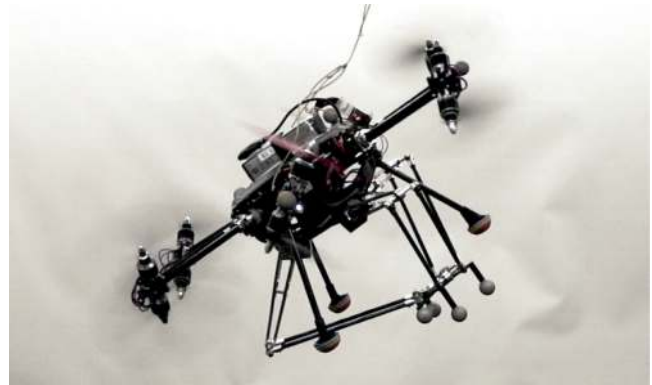
Fig. 1. Omnidirectional delta-based parallel aerial manipulator.
