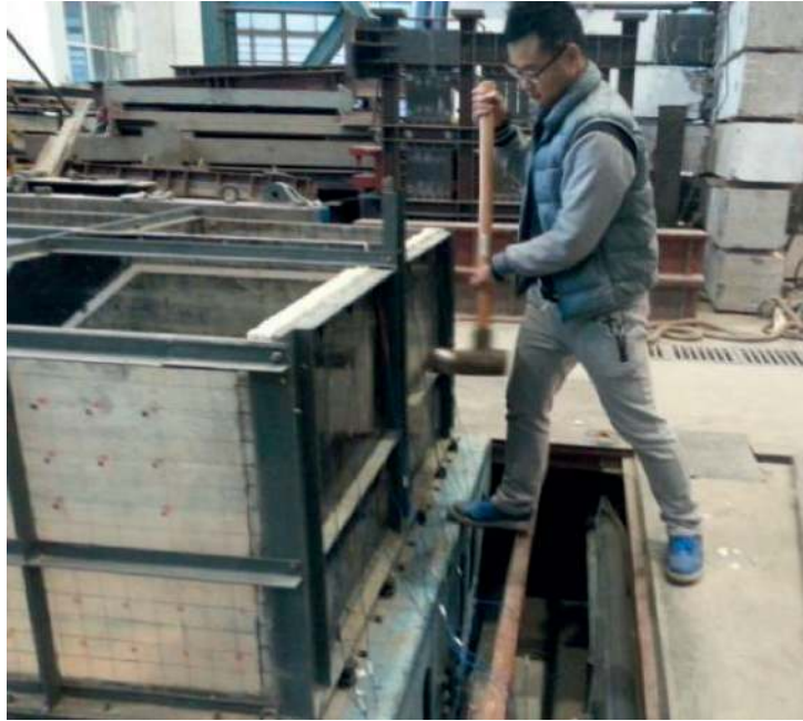
FIGURE 7: Hammer test of model box.
