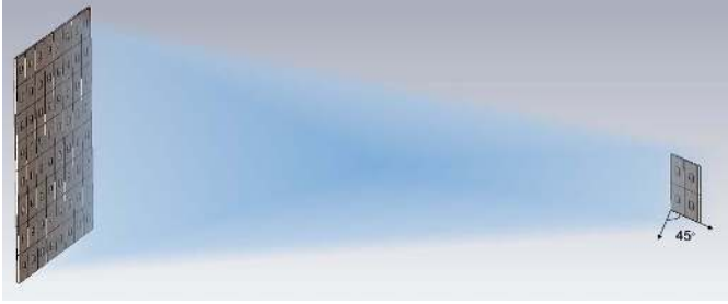
Fig. 1. 8 \times 8 -GU ( G = 64 ) facing a 2 \times 2 -RU ( R = 4 ) at a 45^\circ angle with conceptual field profile under focusing.
