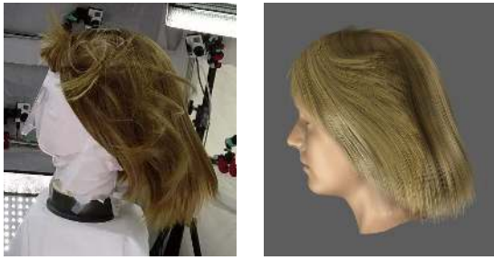
Figure 12: Failure Case: When the hair motion is highly chaotic, our method will produce over-smoothed result.
