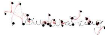
Fig. 2. Dynamic acquisition (“♦”: pen-down; “•”: pen-up; black dots: on pad samples; red dots: on air movement samples)
