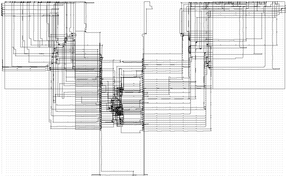
Figure 7: DHP Floorplan of the RAD FPGA. A single module has been routed and placed to fit within the area of one DHP module. Using PARBIT, this DHP can be placed into either location of the Infrastructure shown in the floorplan above. Note that input/output signals are routed to I/O pins so that standard design flows for synthesis and simulation of the FPGA circuit can be followed.
