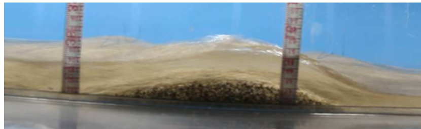
Figure 7 Dynamic hydraulic jump in SPH: (a) without sediment; (b) initial stage of hydraulic jump; and (c) - (e) dynamic hydraulic jump propagates upstream, until 1.4-1.0 m from the inflow boundary
