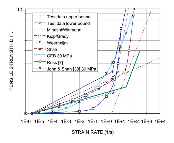
Figure 3. Comparison of various theories and experimental data, adapted from [34].
