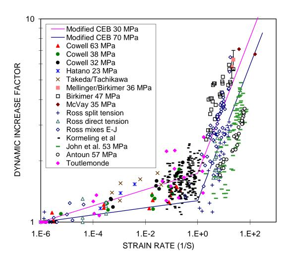
Figure 4. Proposed modified CEB curves in tension.
