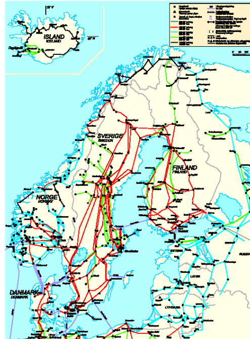
Figure 6.20 High voltage Nordic power network [75].
