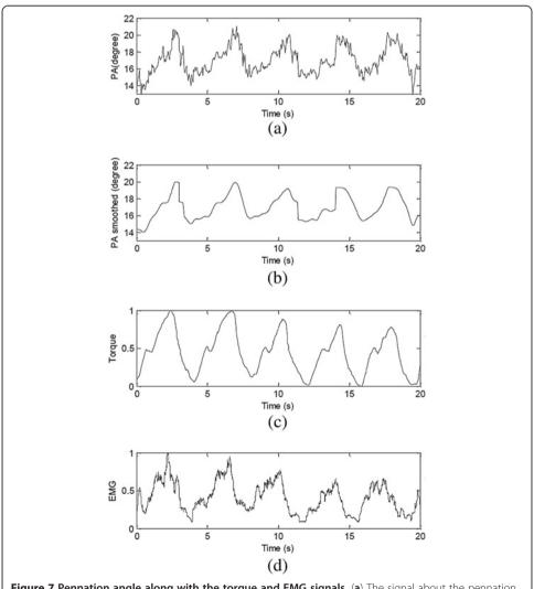
**Figure 7 Pennation angle along with the torque and EMG signals.** (a) The signal about the pennation angle (PA) estimated using the automatic method, (b) Smoothed signal of (a), (c) the torque signal recorded, and (d) the EMG RMS signal.
