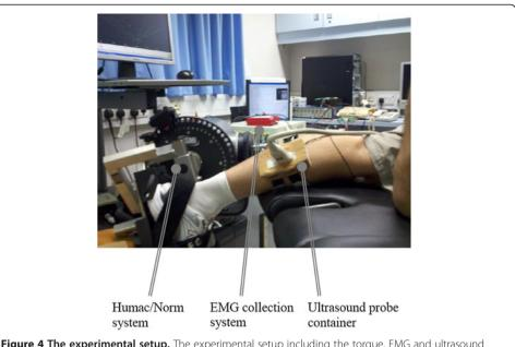
**Figure 4** The experimental setup. The experimental setup including the torque, EMG and ultrasound image data collection modules.
