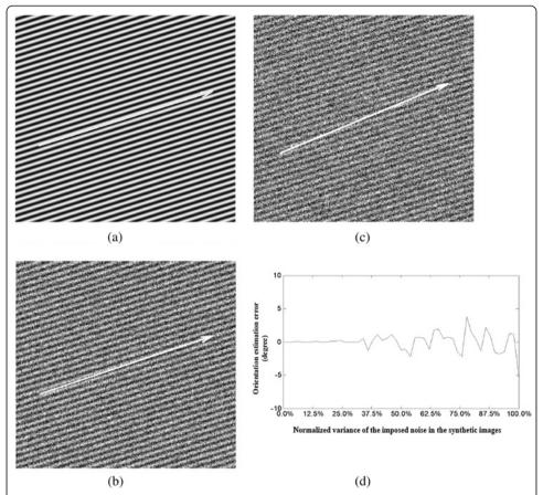
**Figure 3** Analysis of results on synthetic images. Analysis of results on synthetic images with different noise levels, the actual orientation is arctangent of 1/3 (18.4 degrees), the arrows overlaid on (**a-c**) stand for the orientations estimated. (**a**) Synthetic image, noise: mean = 0, normalized variance = 0%; (**b**) Synthetic image, noise: mean = 0, normalized variance = 100%. (**d**) Errors of the estimated orientation compared to the actual value.
