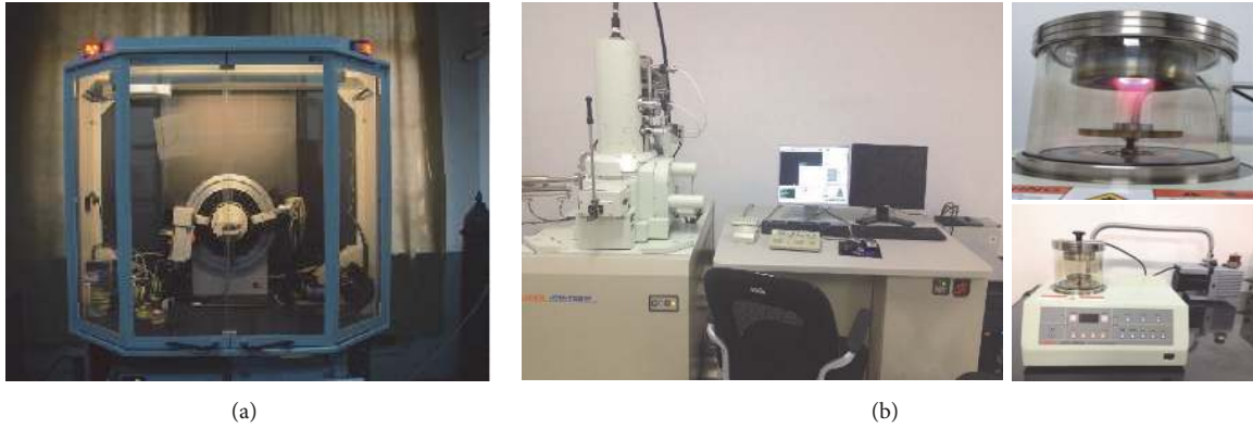
FIGURE 1: D8 Advance X-ray diffractometer (a) and JSM-7001F Field Emission Transmission Electron Microscopy (b).
