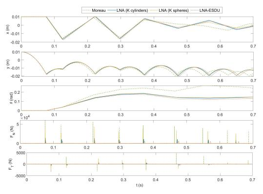
**Figure 8.** Model comparison considering an asymmetrical impact: from the top to the bottom: *x*-coordinate of  $G_1$ , *y*-coordinate of  $G_1$ , rotation angle  $\theta$  of body 1, normal contact force  $F_N$ , tangential friction force  $F_T$ .
