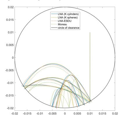
**Figure 10.** Trajectory of the body–center  $G_1$  for the four models considering the asymmetrical impact. Starting point at  $\mathbf{q}_0 = [0.01, 0.01, 0]^T$ .
