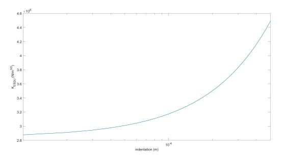
Figure 5. Generalized stiffness evaluated using the Lankarani–Nikravesh/ESDU impact model [22].
