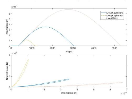
**Figure 7.** Model comparison considering an asymmetrical impact: from the top to the bottom: indentation *vs.* number of steps; hysteresis cycles.
