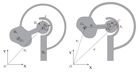
Figure 2. Undeformed CSFH (left). Deformed CSFH with impact (right).
