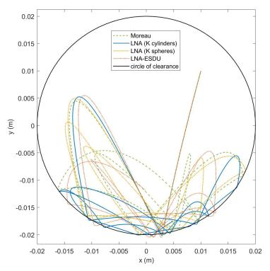
**Figure 12.** Trajectory of the body–center  $G_1$  for the four models. Starting point at  $\mathbf{q}_0 = [0.01, 0.01, 0]^T$ .
