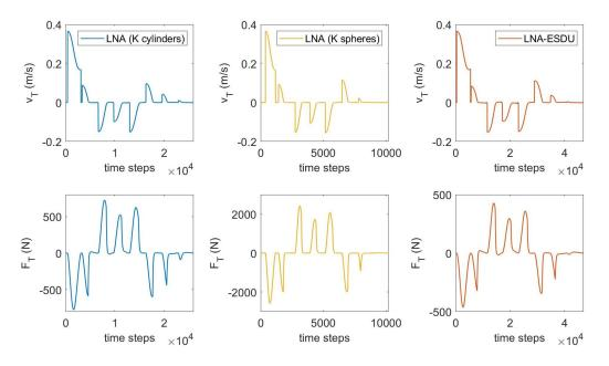
**Figure 9.** Relative tangential velocity  $v_T$  and friction force  $F_T$  in terms of the number of time steps.
