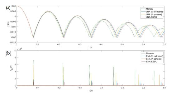
**Figure 6.** Model comparison considering a central impact: (a) *y*-coordinate of  $G_1$ , (b) impact force  $F_N$ .
