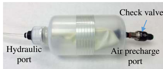
Figure 17. Ballast tank design with precharge port
