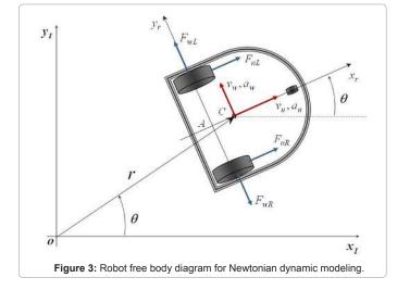
We start the derivation by representing the robot position using polar coordinates. Assuming that the robot is a rigid body, its polar coordinates in the inertial frame can be represented using a complex vector
