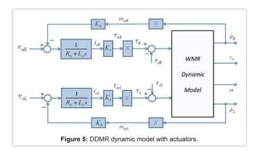
are obtained by combining equation (76) for each motor with the mechanical dynamics of the DDMR. Additional torque disturbances acting on the wheels can be included as additive terms to the motor torques. Figure 5 shows a block diagram representation of the overall system. The forward kinematic model (19) can be added as a cascade to the dynamic model to form a complete model for simulation and analysis of the DDMR.
