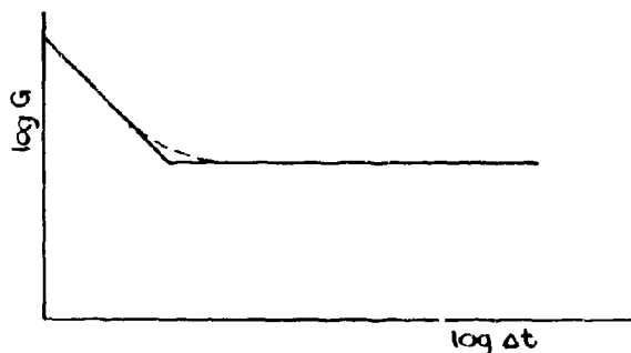
Figure 11. A Tolerance Graph for Rectangular Pulse Inputs.
