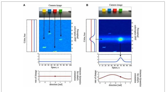
FIGURE 2 | A small DNF architecture, which consists of a two-dimensional color-space DNF (center), one-dimensional color- and space- DNFs, coupled to the perceptual DNF, a camera input (top), and an attractor motor dynamics (bottom). (A) The camera input alone is not sufficient to activate the perceptual DNF, the system is quiescent and produces neither output nor behavior. (B) A color cue creates an activity peak
