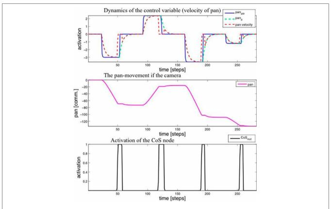
FIGURE 7 | Top: Time-course of the activation of the motor variable (velocity of the pan joint) during four steps of the learning procedure. **Middle**: The value of the pan variable. **Bottom**: Activation of the CoS node.
