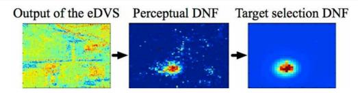
FIGURE 5 | The cascade from the visual input to perceptual DNF to the visual intention (target) DNF segregates and stabilizes the selected region in the input stream.
