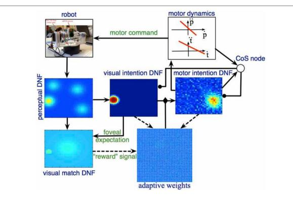
**FIGURE 6 | The DFT architecture for autonomous looking and learning the sensorimotor map.** The robotic camera provides input to the perceptual DNF, which performs initial segregation of object-like regions in the visual stream. The visual intention DNF selects and stabilizes the spatial representation (in visual coordinates) of a single target for the upcoming looking action. Through adaptive weights, the visual intention DNF provides
