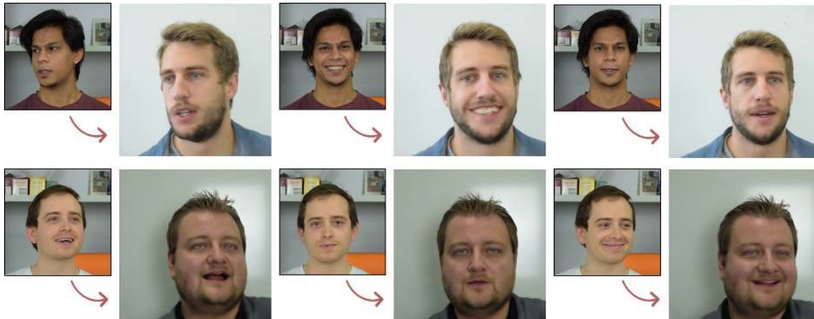
Figure 7: Our 4D facial avatars allow for facial reenactment, where the expressions of a source person are transferred to a target actor which we represent with our dynamic neural radiance field. Note that for facial reenactment we only need to train a model for the target actor; the expressions and pose changes from the source actor can be obtained in real-time [41].
