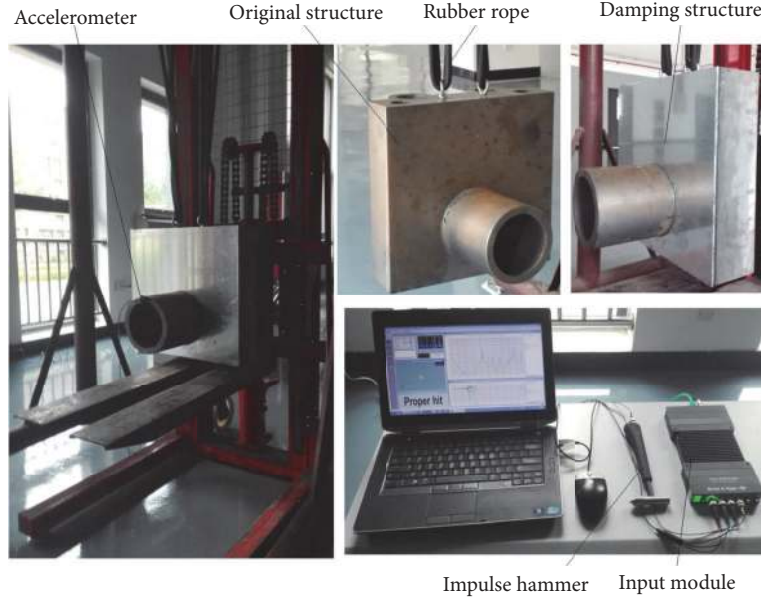
FIGURE 13: Experiment setup of the headstock.
