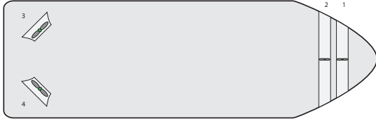
Fig. 3: Thruster layout of the simulated vessel, with two tunnel thrusters near the bow two rotatable azimuth thrusters at the stern. The thruster numbers are shown.
