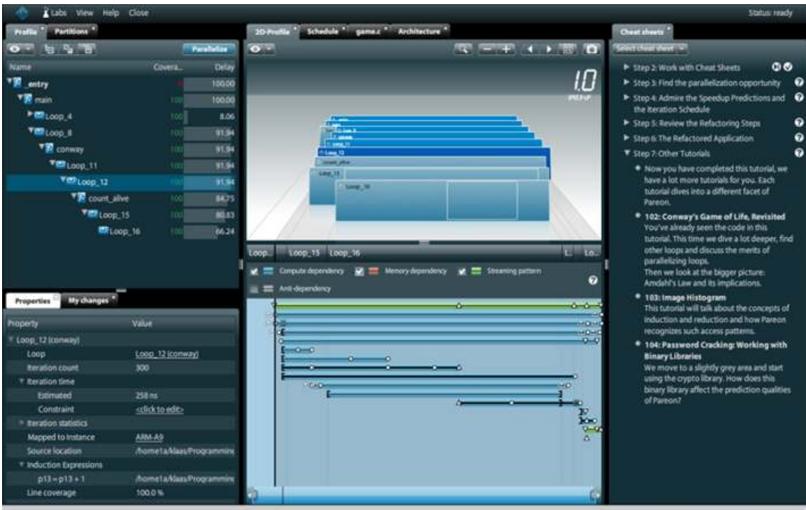
Figure 20: Vector Fabrics Pareon (formerly vfThreaded x86): A graphical user interface to show loop-carried dependences.
