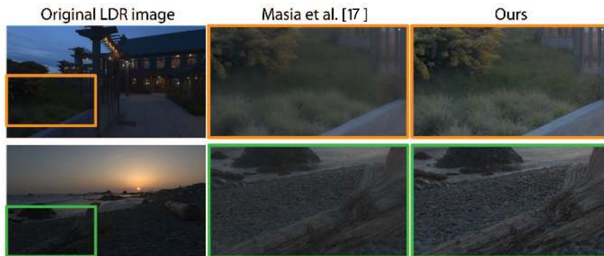
Fig. 9 Original LDR image and a cropped region of the tonemapped result of the expansion with the \gamma obtained in [17] and our \gamma . Top row: McKeesPub ; bottom row: Redwood-sunset [13]. Note the increased contrast yielded by our method. Please refer to the digital version of the article for full appreciation of the details
