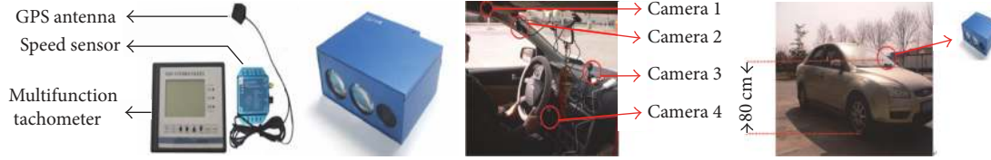
FIGURE 3: Dynamic Driver-Vehicle-Environment information acquisition system.
