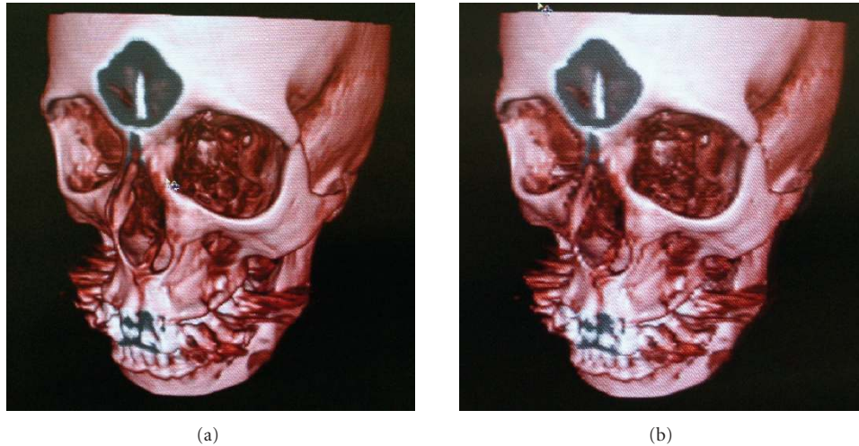
FIGURE 10: (a) The lenticular screen has been photographed to show how a view is being displayed, rendered at the 1/3 orthogonal grid resolution. (b) The same view, but sampled at 0.375 the resolution of the view in (a). Though the downsampling is visible, the effect is less strong than might be expected. This can be contributed to the fact that the displaying process possesses a low-pass filter character, due to effects like crosstalk.
