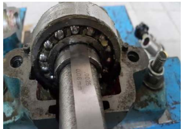
Fig. 5 Clearance of 0.02 mm in the sleeve and inner race
