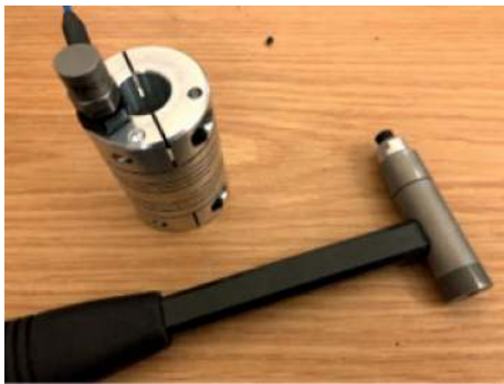
FIGURE 7: Experimental procedure used to find the coupling's damping values.
