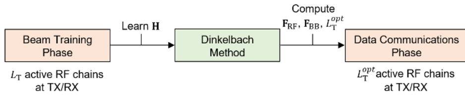
(b) Block diagram of the beam tracking phase and the data communications phase.
