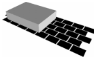
Fig. 3. 3D rendering of the complete model showing a 1.15 \times 0.4 \times 0.25 \mu\text{m} , 550 \mu\text{g} part resting at its initial position over an 8 \times 5 resonator array.
