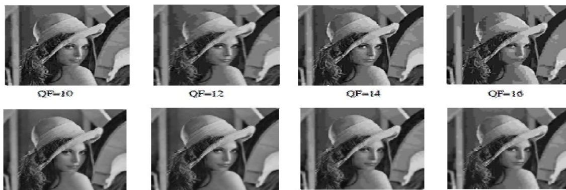
Fig. 3: Upper row is reconstructed Lena image using DCT based compression. Below is blocky artifacts reduction using proposed DCT and DSR based technique
