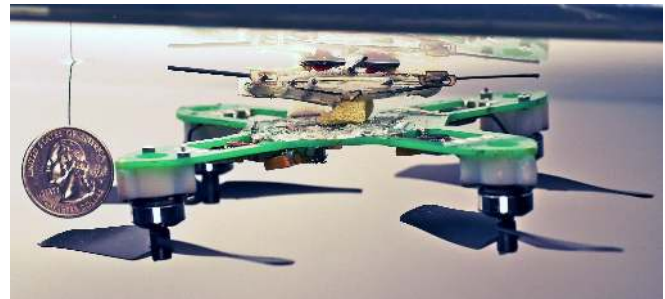
Fig. 1. Quadrotor Micro Air Vehicle hanging from a glass surface using the directional adhesive Collapsing Truss Grasper (Sec. III-A).
