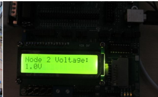
Fig.7 LCD display of master displaying ADC voltage of node 2.
