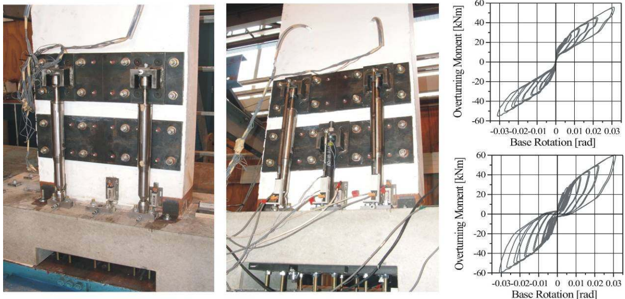
Figure 10: As-built wall units; Left: Unit 2 (4 viscous dampers), Centre: Unit 3 (4 viscous dampers and 2 TCY mild steel dampers), Top Right: Experimental response of HY_{2MS-0V} (testing at 0.5Hz frequency), Bottom Right: Experimental response of HY_{2MS-4V} (testing at 0.5Hz frequency).
