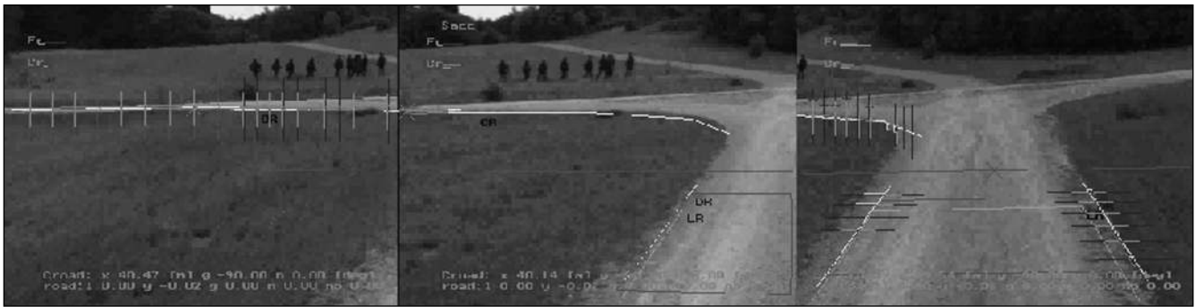
Figure 10. Teleimages during Saccadic Vision When Approaching a Crossroad. The center image during a saccade is not evaluated (missing indicated search paths).
